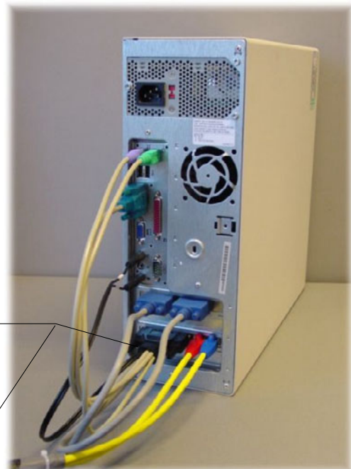
WS-Remote PCI dual card with special connector for USB, Audio and 2 Video outputs.
